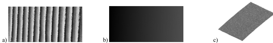
Fig. 2 Experimental results for normal displacement measurement of a tilted plane with a phase grating at \lambda = 785 nm a) wrapped phase map; b) unwrapped phase map; c) 3D presentation
