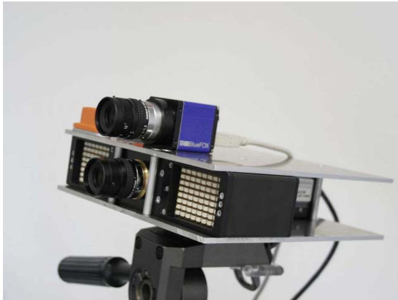
Fig. 9. SAD – Our scene acquisition device for 3D content – e.g., for 3DTV
