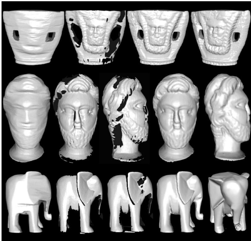
Fig. 16. (Cup object, first row) Silhouette reconstruction, optical triangulation reconstruction, and two views from the model obtained by fusion, respectively. (Head object, second row) Silhouette reconstruction, two views from optical triangulation reconstruction, and two views from fusion. (Elephant object, third row) Silhouette reconstruction, optical triangulation reconstructions from two separate scans, and two views from fusion.
