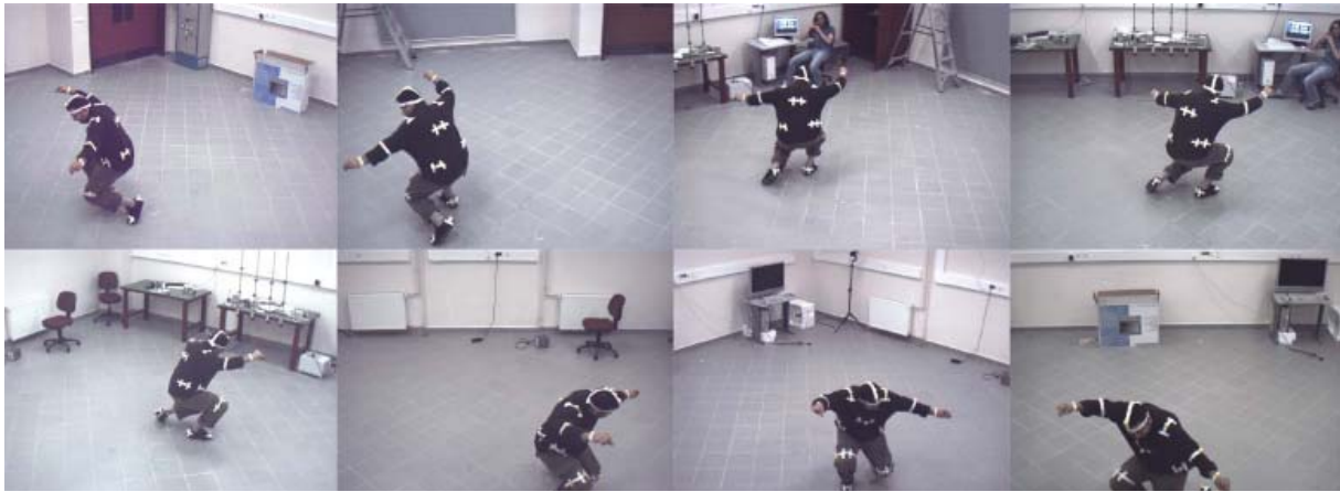
Fig. 17. Dance scene captured by the 8-camera system available at Koc, University. Markers are attached at or around the joints of the body.
