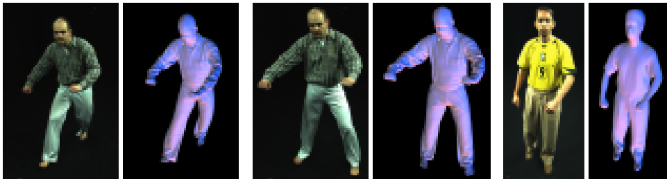
Fig. 22. Our framework correctly tracks 3D trajectories of features over time. By combining the 3D point trajectories with our mesh deformation method, our algorithm is able to directly animate a human body scan.
