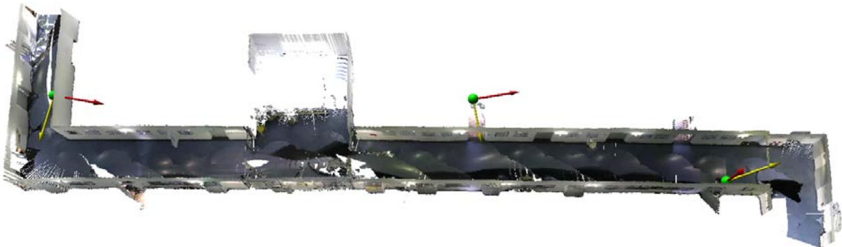
Fig. 15. Underlying model used in the self-localization process. The model shows our department main floor, acquired by our Wägele model acquisition platform. Observer camera frames (reference and up vector) are visualized.
