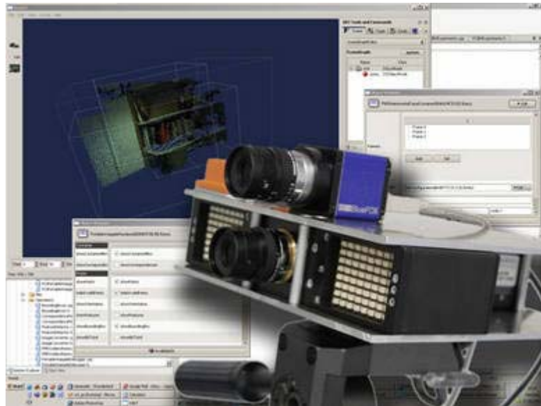
Fig. 8. SAD Multisensor Scene Acquisition Device
