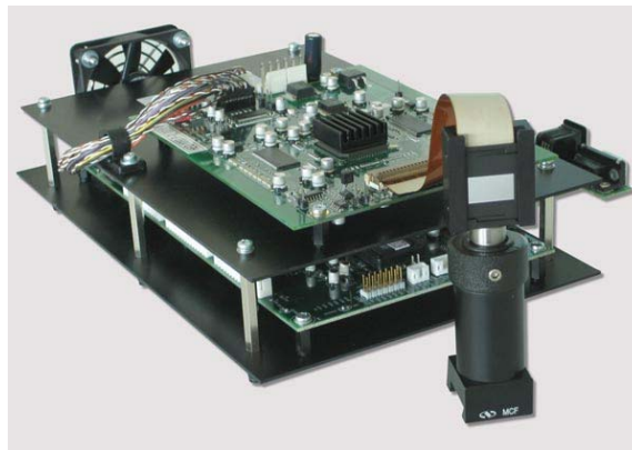
Figure T5-3 Holoeye HEO1080P LCoS SLM [after 2]
